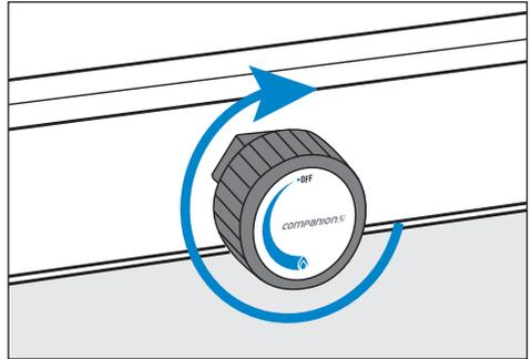
Turn the gas controls to the OFF position.
