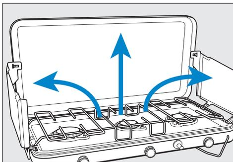
**Step 2.** Select the burner to be ignited and slowly turn the gas control in an anti-clockwise direction approximately  $\frac{1}{4}$  of a turn.
