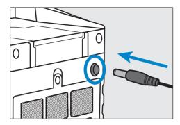
**Step 1.** Ensure unit is switched off prior to charging, installing or replacing battery.
