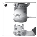
4. Insert pot trivot, with legs folded into pot, attach lid, lock in place and store
