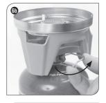
(c) Press the Piezo until the burner lights **Note:** If Burner does not ignite, turn the gas supply off and wait for excess gas to disburse before repeating the lighting process
