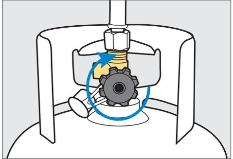
**Step 1.** With the flame still operating, turn the valve on the gas cylinder in the clockwise direction until it is OFF. Allow the flame to burn down then extinguish once all remaining gas in the hose has been used.
