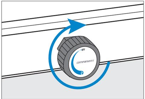
**Step 2.** Turn the gas controls on the appliance clockwise to the OFF position.
