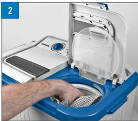
**Step 2.** Place a selection of articles in the spinning tub and insert the spin disc.
