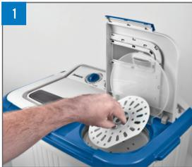
**Step 1.** Open the External and Internal lids of the spinning tub and remove the plastic spin disc. Note: It is important that the spin disc is used every time so as to allow correct operation of the spinner tub.
